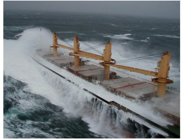
Figure 4 A bulk carrier outbound over the Columbia River Bar. Deployment and retrieval of GPS equipment on deck is not practical under such conditions. To capture such conditions an alternative ship motion measurement approach is required. Photo courtesy of Columbia River Bar Pilots.
