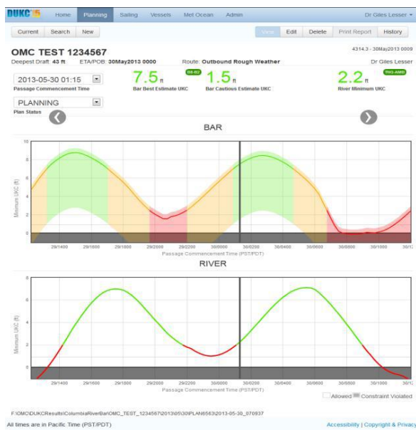
Figure 6 Example planning output of the demonstration DUKC® system for the Columbia River Bar showing 24 hour scans of predicted UKC over both the Bar and River sections of the transit for a particular ship. Red, orange and green indicate times of high, medium and low risk of grounding respectively.
