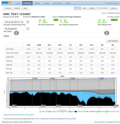
Figure 5 Example output of the demonstration DUKC® system showing a profile of UKC-related information for a particular transit of a specific ship. Black indicates sea bed, light grey is ship’s draft and dark grey is dynamic motions allowance. Pale blue indicates predicted UKC.
