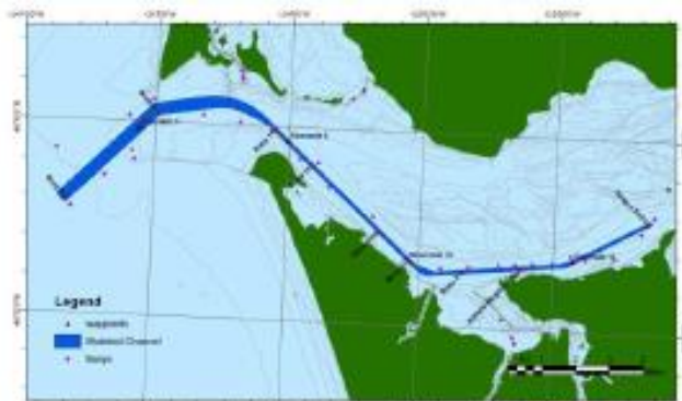
Figure 3 Arrangement of the DUKC calculation locations for the Columbia River Bar. Calculation locations are arranged every ¼ mile (400 m) along the deep-draft shipping channel. This layout provides sufficient resolution to capture spatial variation in ship keel elevation while keeping computational effort to a manageable level.
