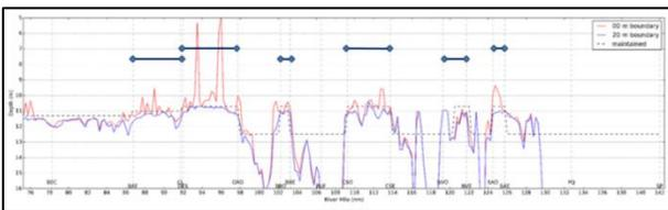
**Figure 11: Graph of along channel bathymetric depths. Shallower sections are defined as legs with gates either side.**
