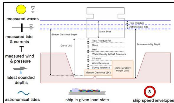
Figure 5: Schematic of the various factors that influence UKC.
