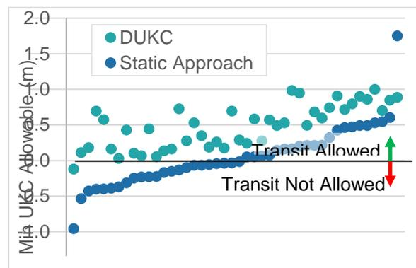
Figure 6: Comparison of DUKC and Static UKC rules for 44 actual deep draft transits. A dot below 0.0 m indicates that transit broke either the Static UKC rules or the DUKC rules. No transit actually grounded.
