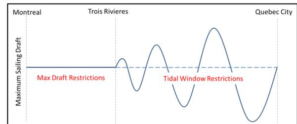
Figure 3: Schematic of draft limits for vessels transiting between Port of Montreal and Quebec City.
