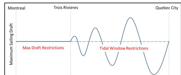
Figure 3: Schematic of draft limits for vessels transiting between Port of Montreal and Quebec City.
