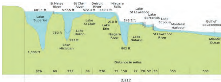
Figure 1: The cross section of water levels and depth of various components of Great Lakes/St. Lawrence system.
