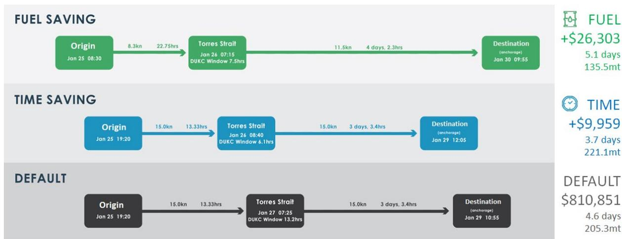
Figure 4 – Presentation of Berth to Berth alternate suggestions for voyage scheduling for a specific draft target; the schedule timing alternatives for a given draft are visually contrasted in time and financial terms; fuel and time are balanced in financial terms (cargo versus draft can also be balanced)
