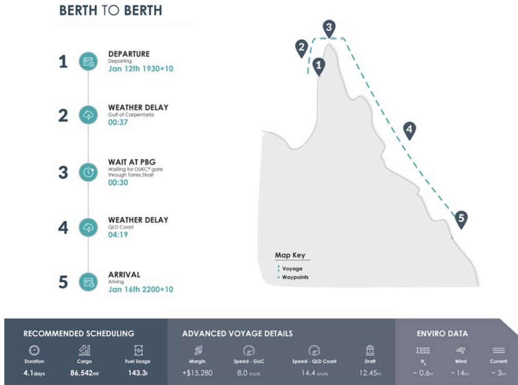
Figure 1 – An example of Berth to Berth voyage schedule advice displayed as an infographic; the overall advice is visible at a glance with details available in the bottom bar; this user experience provides ease of use for schedulers
