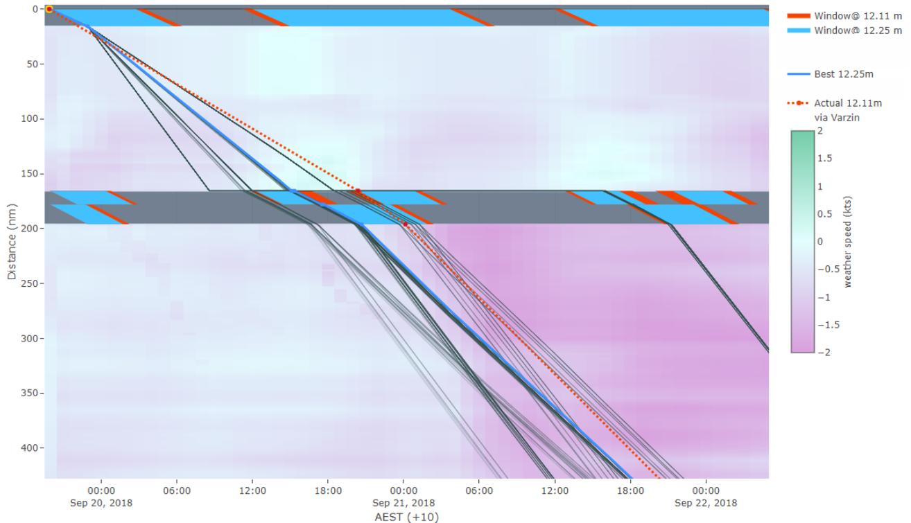
Figure 5 – A prototype system screenshot where alternate scenarios are compared taking DUKC(R) windows; vessel speed characteristics and forecast weather into account; the weather impact on speed and fuel efficiency over the south-bound leg can result in divergent strategies for optimal outcomes
