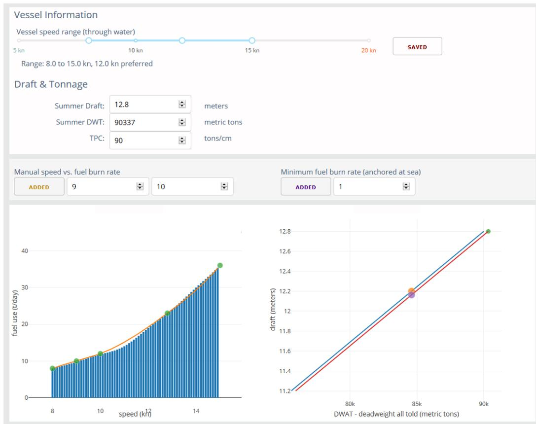
Figure 3 – Screenshot of prototype system vessel particulars input & display; fuel consumption curves can be inferred from few data points or fully entered, and draft-tonnage characteristics are loaded from a database; these ship characteristics can be vital in determining optimal strategies since these characteristics determine the financial outcomes
