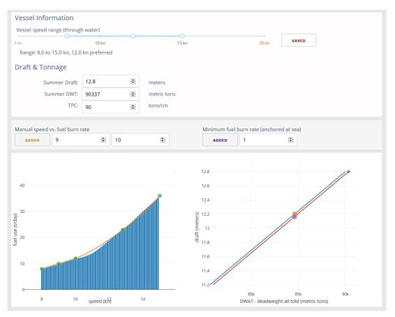
Figure 3 – Screenshot of prototype system vessel particulars input & display; fuel consumption curves can be inferred from few data points or fully entered, and draft-tonnage characteristics are loaded from a database; these ship characteristics can be vital in determining optimal strategies since these characteristics determine the financial outcomes
