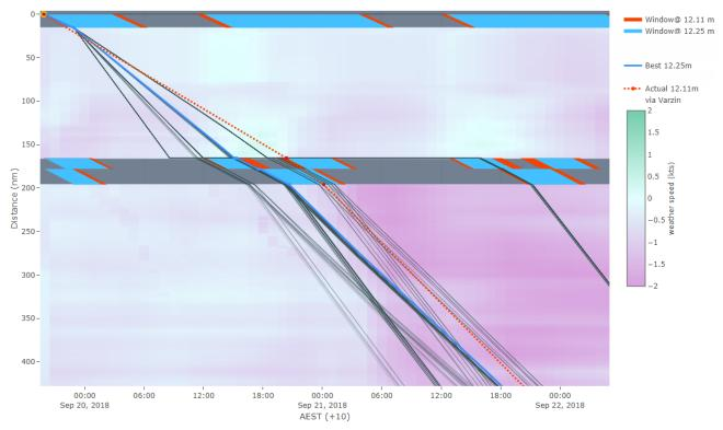
Figure 5 – A prototype system screenshot where alternate scenarios are compared taking DUKC(R) windows; vessel speed characteristics and forecast weather into account; the weather impact on speed and fuel efficiency over the southbound leg can result in divergent strategies for optimal outcomes
