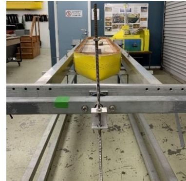
Figure 2. Marad F model on the roll frame
