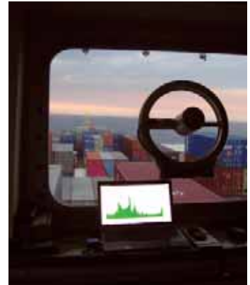
DUKC system from OMC monitors under keel clearance
