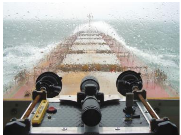
Figure 4 - iHeave recording vessel motions while mounted on wheelhouse windscreen (image courtesy of the Columbia River Bar Pilots)
