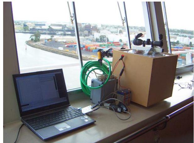
Figure 5 - prototype iHeave testing through Port of Melbourne waterways
