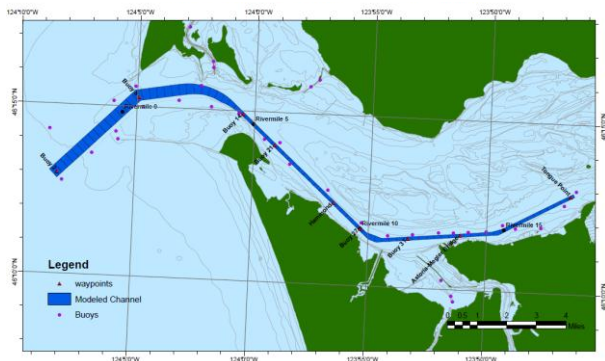
Figure 3 Arrangement of the DUKC ® calculation locations for the Columbia River Bar. Calculation locations are arranged every ¼ mile (400 m) along the deep-draft shipping channel. This layout provides sufficient resolution to capture spatial variation in ship keel elevation while keeping computational effort to a manageable level.
