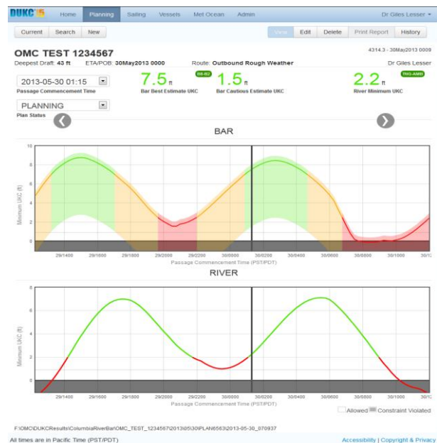
Figure 6 Example planning output of the demonstration DUKC® system for the Columbia River Bar showing 24 hour scans of predicted UKC over both the Bar and River sections of the transit for a particular ship. Red, orange and green indicate times of high, medium and low risk of grounding respectively.
